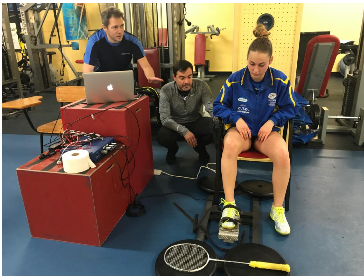
Picture 1 – Experiment set-up used to assess voluntary/explosive strength production capacity in the plantar flexors and dorsi flexors.
