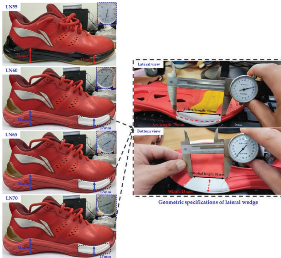
Figure 1. Illustration of LN55, LN60, LN65, and LN70 badminton footwear specifications, with an arc length of 75mm (lateral midsole wall), lateral length of 72mm, medial length of 51mm, and width of 23mm.
